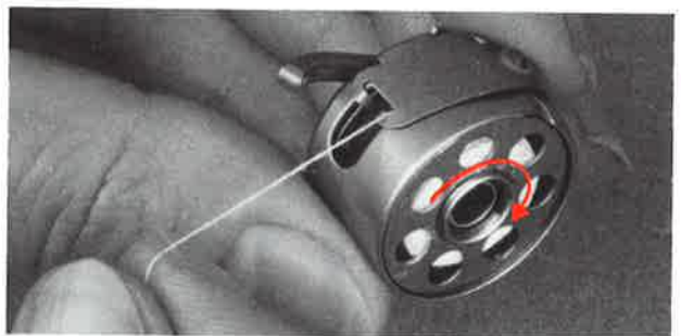
▲9 Pull the thread under the spring until it lies in the T-shaped slot at the end of the spring.
